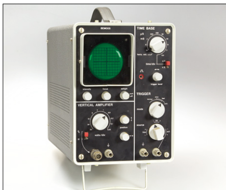
Figure 7. The BEM005 oscilloscope. Note again that this instrument was built from a kit of parts.
