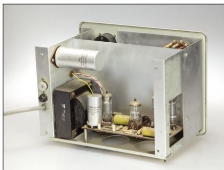
Figure 5. Inside the BEM004: conventional construction techniques using vacuum tubes, and a chassis.
